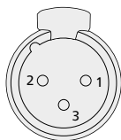
DMX-OUTPUT XLR mounting-sockets (rear view)
